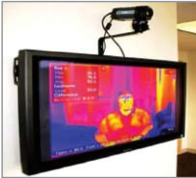
Fixed-mount A320 w/full thermal imaging on video monitor.
