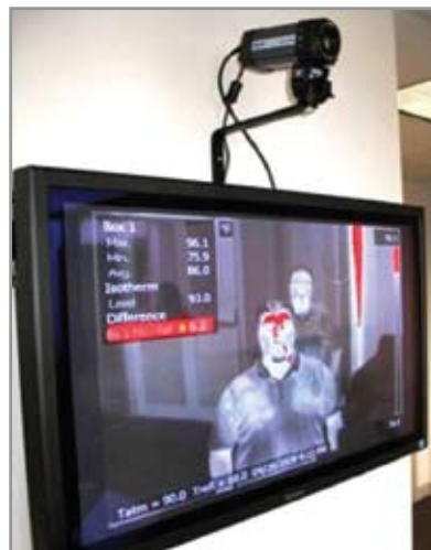
Fixed-mount A320 w/full thermal "color alarming" in progress.
