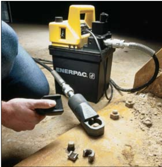
▲ Enerpac Nut Splitter being used to remove the nuts holding on a bucket edge on a skid steer loader
