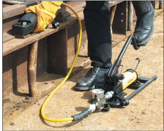
▲ Easily removing rusty nuts during railroad construction is just one of many application examples for the Enerpac Nut Splitter.
