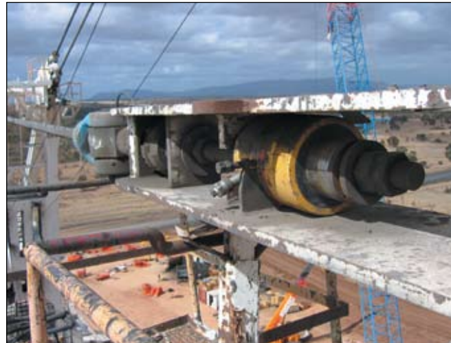
Hollow plunger cylinder RCH-1003 used in an application for intermediate boom suspension on a dragline.
