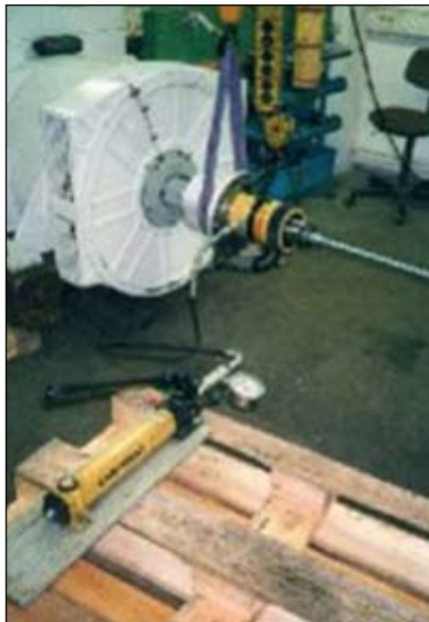
5ZL54 hollow plunger cylinder being used to press the coupling on the shaft of a turbine
