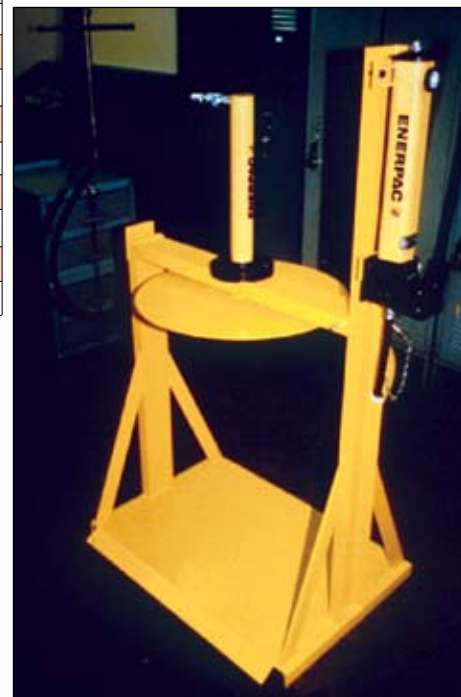
▲ Waste barrel press constructed using an Enerpac hand pump and an RC-series cylinder. When force is applied with the hand pump, the Cylinder presses the top plate down to compress waste in barrels.
