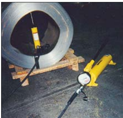
▲ Using an RC-series cylinder to correct the central eye of a roll of steel which was compressed during transport
